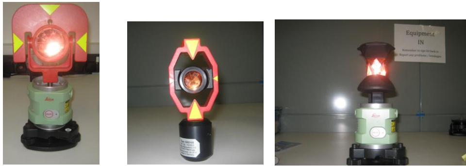
Fig. 2: (a) Leica GPR111 (b) Leica GMP111 (c) Leica GRZ4 target
