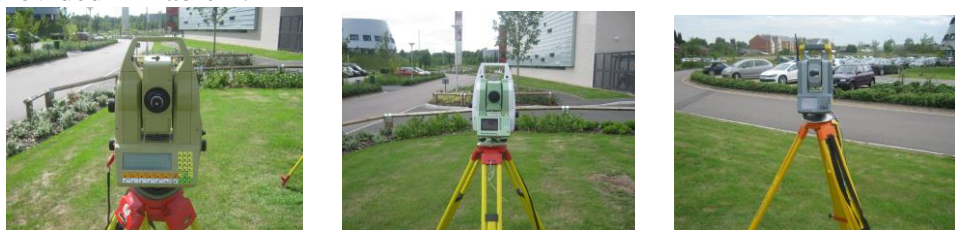
Fig. 1: (a) Leica TCA2003 (b) Leica TS30 (c) Trimble S6 total stations
