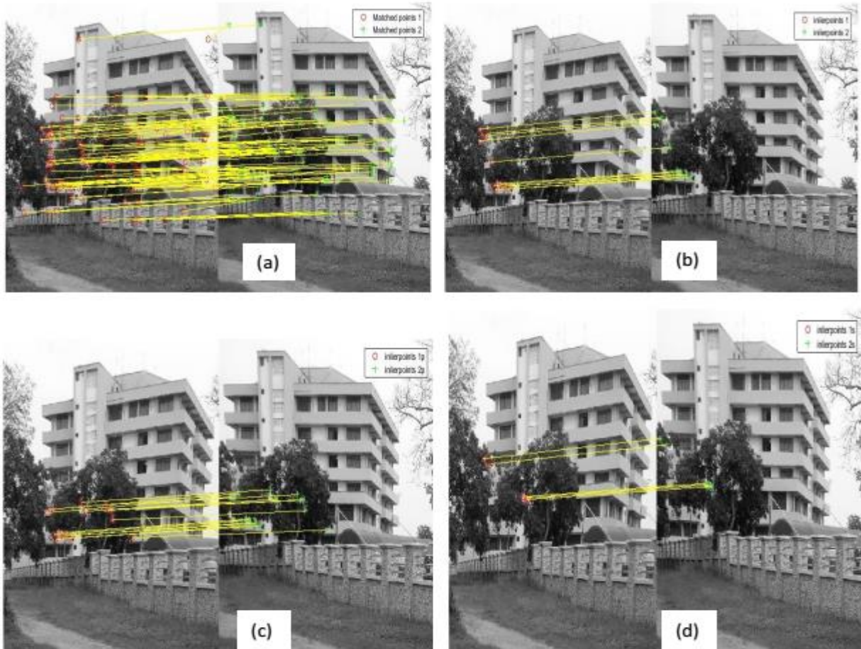
Figure 4: Detection and elimination of type II errors by tree transforms: (a) Set of matched points containing 50% type II errors and 50% correctly matched points (inliers). (b) Detected inliers after eliminating type II errors using Affine transform. (c) Detected inliers after eliminating type II errors using Projective transform. (d) Detected inliers after eliminating type II errors using Conformal transform.
